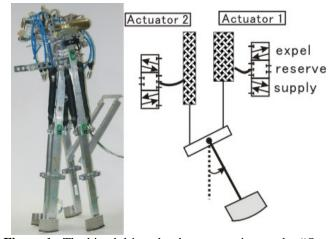
**Figure 1**: The biped driven by the pneumatic muscles "Quekaku" (left) and the schematic construction of the joint driven by the antagonistic pair of muscles (right).
